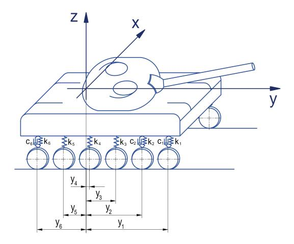
Fig. 3. Schematic diagram of the tank suspension
