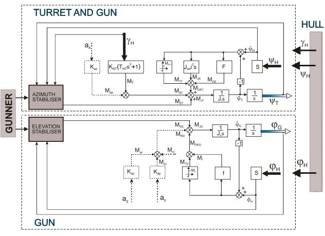
Fig. 2. Structural scheme of stabilised main armament
