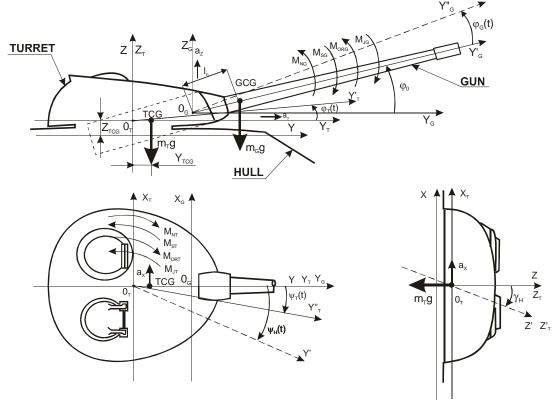
Fig. 1. Main moments and forces acting on the turret and the gun of the tank
